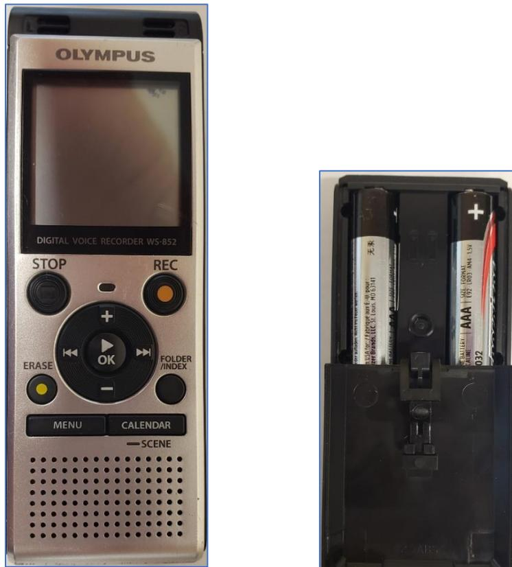
To begin, turn the device on by finding the slider on the right side of the device, labeled **POWER**. Push the slider up to the **ON** position.
