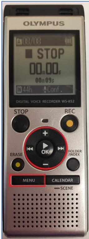
3. Use the up and down buttons (+/- above and below the OK button) to move through the menu and select **"Device Menu"**. On this new menu, move to **"Time & Date"**.
