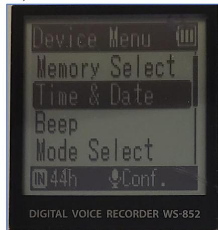
4. Check this screen to see if the date and time are correct. If they are not, use the side keys (left and right of the OK button) to move between month, day, year, and time, and use the up and down buttons to change each one. When the date/time is correct, press the center “OK” button.
